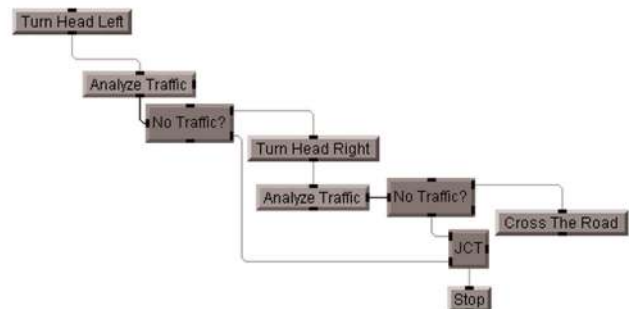
Figure 3: Dependency of sub-tasks in a program to control a robot using Keysight VEE
