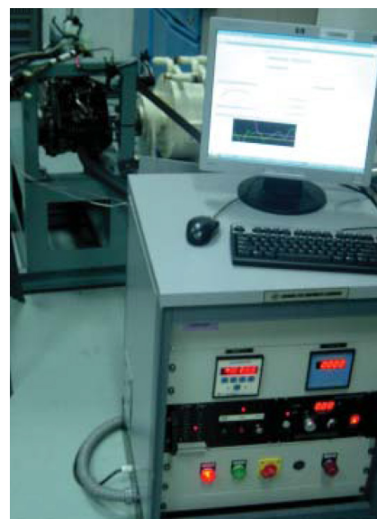
Figure 6. Controller in the foreground, engine and dynamometer behind
