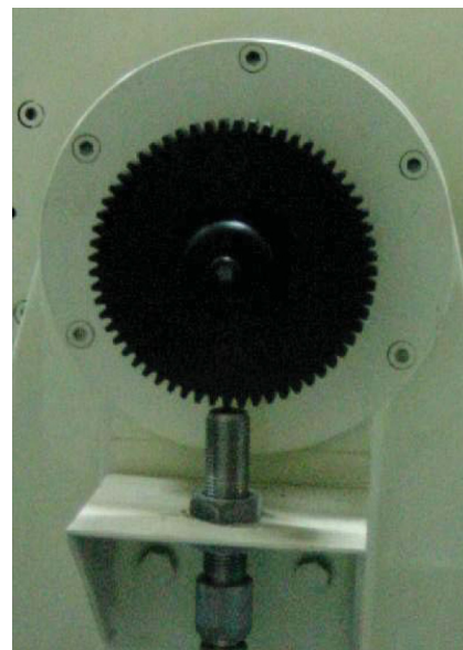
Figure 4. Speed wheel (top) and pickup (below)
