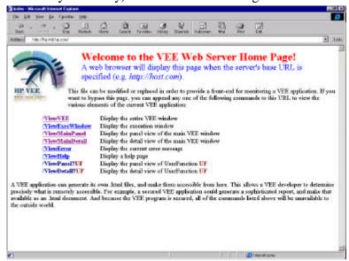
This web page defines the commands that the VEE web server will accept. So you can navigate the VEE program by clicking on the appropriate command on the web page shown above, or directly type in the URLs as:
