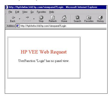
If an engineer wants another to see his programming code, those viewing the HP VEE program can access the code of the Main program or any User Functions by using the ViewMainDetail command or the ViewDetail?UserFunction command. Below is an example of User Function called "Login" from the manufacturing test example from above. The user types in: <a href="http://hp.lvld.hp.com/ViewDetail?Login">http://hp.lvld.hp.com/ViewDetail?Login</a>:
