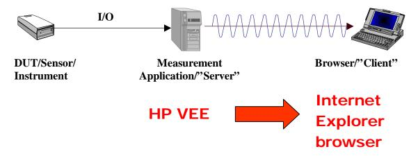
HP VEE 5.0 has the ability to allow a browser to see the view from parts of a VEE program, which means it has a built-in web server. When the designer wants to enable the server in HP VEE to allow data to be viewed, he will enable it via the new "**Web Server**" tab in Default Preferences dialog box. HP VEE must be running on a system that is connected to a network for the web feature to work.
