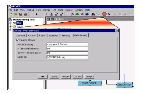
If HP VEE 5.0 is installed on a Win95/NT operating system with the default suggestions, this field will read "C:\Program Files\Hewlett-Packard\VEE 5.0\www." By changing the HTTP port the server "listens on" from the default of 80, you can limit who can see the data as only they will know the correct port on which to send the data from their browswers. For instance if port 91 were chosen the user would use the following URL: <a href="http://hostname:91">http://hostname:91</a>.
