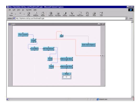
As you can see, this allows several engineers to troubleshoot code remotely by looking at the details of the HP VEE program code loaded on another machine.
