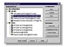
HP VEE 4.0's Instrument Manager scans the bus for devices and automatically handles the interfacing details, so you no longer need to build address strings, load drivers, and manage I/O session handles.
