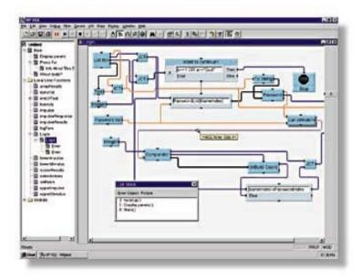
The Program Explorer helps you navigate through complex programs, both during debug and after the test program is up and running.
