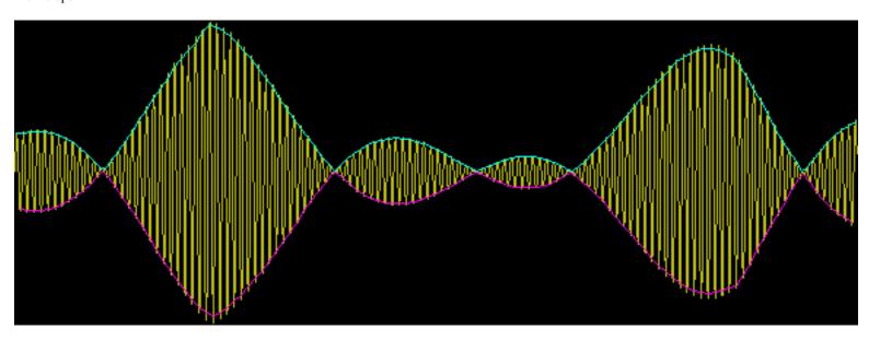
o\_envelope(A,3) returns minima using Method 2 o\_envelope(A,0) returns maxima using Method 1
