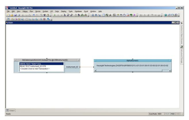
If successful, the VEE program starts with the *Direct I/O* object which will write the identification query ("\*IDN?") out to your instrument and read the identification string from your instrument. This identification string is passed to the *AlphaNumeric* display object and the VEE program stops.
