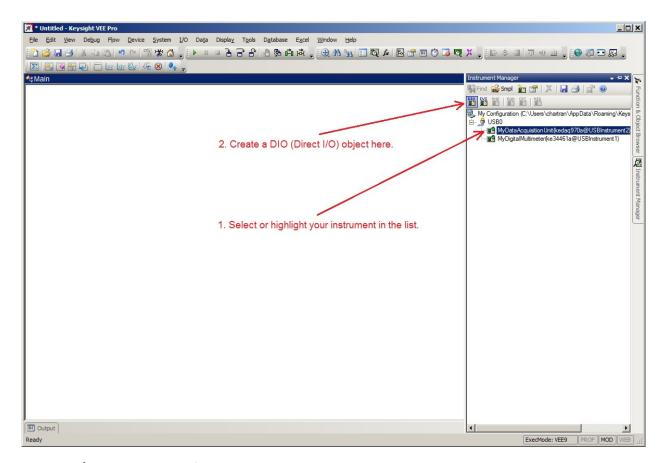
A *Direct I/O* object is shown for your instrument on the VEE whitespace below. This object is used to write IEEE-488.2 common commands, SCPI commands, or SCPI queries <u>directly</u> to your instrument. Responses from your instrument can be read <u>directly</u> by this object.
